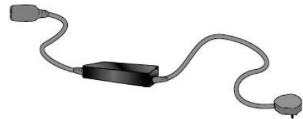
External power supply mounted in cable
