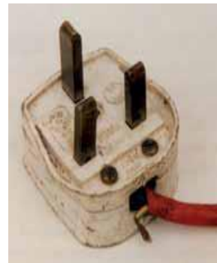
Damaged cable sheath
